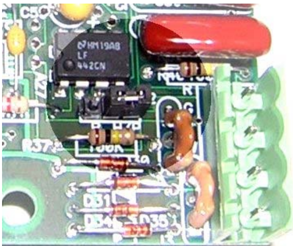
Figure 8.5.1 Jumper setting: Primary Sensor or Hall-Effect Sensor (two pins on the right)
